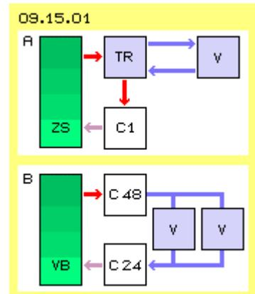
Below at this picture at B, the general principle of that new 'booster-conception' is sketched. From a charge-source of low voltage (C24, white), the current is guided into the 'volt-booster' (VB, green), where the voltage rises up and the current respective charge is shifted into a high-voltage-storage (C48, white). The following current for balancing the voltage-difference is usable for consumers (V, blue).
