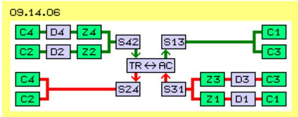
A trafo functions based on increasing and decreasing currents into contrary directions. So the dislocation of charges from C3 to C4 (third row) and from C1 to C2 (forth row) should run through the transformer at opposite ways (here from right to left). So the generated secondary current will be AC. This is the normal mode of a trafo (TR-AC), here driven by displacement of charges in alternating directions.
