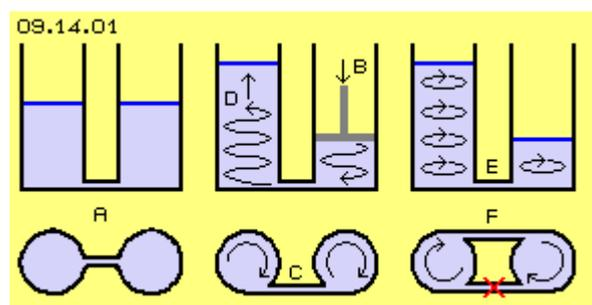
tanks. At B, a piston (grey) presses down the water of the right tank, so the water-level of left tank rises up correspondingly. The 'obtuse' pipe-connection at A would result much resistance. If however a tangential connection C is used, the water can flow off the right tank without resistance. Within both tanks comes up a turning movement. The additional water can enter and 'screw-up' with the turning motion of the left tank by minimum resistance.
