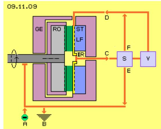
For starting the system, the rotor must be charged from an external source (A), e.g. by gliding-contact at the shaft. For stopping the system, the charge must be allowed to flow-off to the ground (B). This system might become self-accelerating. So that switch for discharge must be installed at any case.
