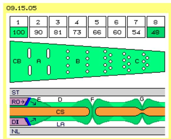
Left side at this picture is drawn a part of the rotor (respective the dielectricum, RO and DI, violet), moving to right side (see arrow). It's frontside should be 'plough-shaped' and build by metal (blue), like discussed at previous chapter: this constructional element rotates within an area filled up by charge and it's gliding along charged storage-faces all times. Soon it will
