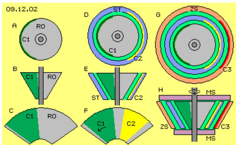
the surface moves increasing faster within space. The elements can be longer stretched at the cone-surface than at the disc-surface. Picture 09.12.02 upside at A shows a view onto the wide side-face of a cone-rotor (RO, grey). A side-view is sketched at B and the outside face is drawn at C.
