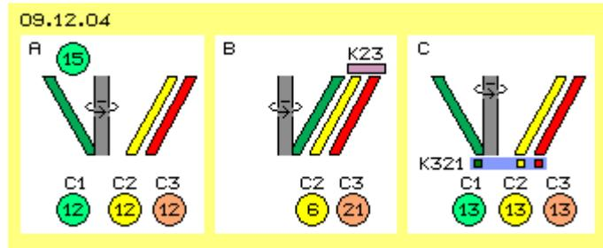
At B the rotor did turn by 180 degree, so now its charge-face covers the stator-face. Their charge-layer (C2, yellow) now is compressed and represents e.g. only 6 V. At upper part with the increased voltage, the rotor-charge affects even stronger pressure respective the charges are faster 'swirling'. The voltage of intermediate storage (C3) thus corresponds not only to previous 18 V, but 3 V stronger, thus showing 21 V.
