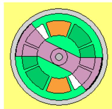
This picture right side shows schematic longitudinal cross-sectional views through the system. The cross-sections of the storages are here not drawn round but rectangle with round edges. The charge respective current can still run around. This construction allows wider storage-surfaces by relative small volume of the housing. The calculations of previous chapter are repeated for this example at the following.
