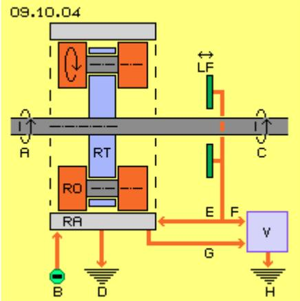
is stored within a housing, however no electric contact exists between these constructional elements and the housing (the housing is not drawn here). The red lines and arrows at this picture represent electric conductors. Depending on phase of operating mode, alternative currents are flowing at these conductors.
