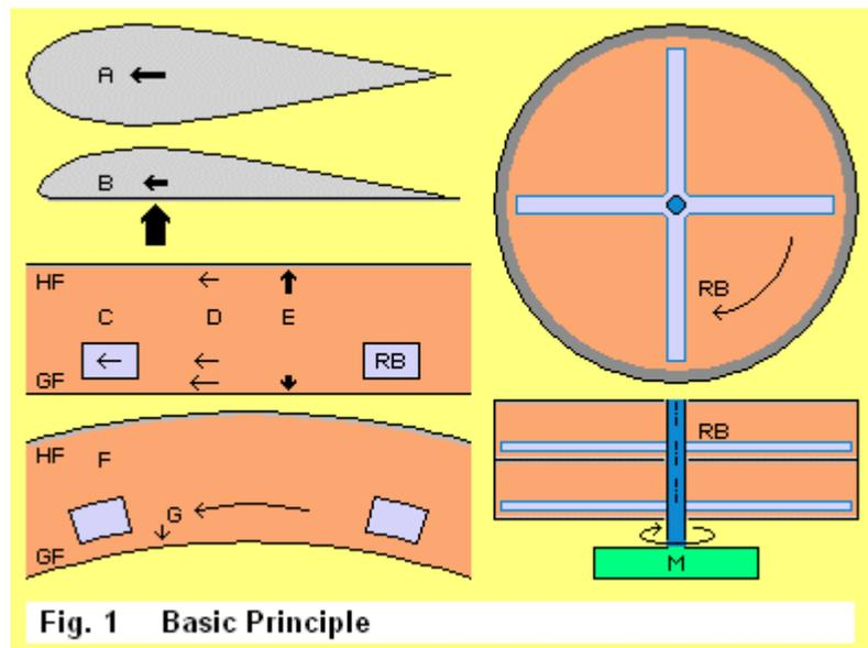
The motion process is comparable with a tracked vehicle. A chain link is laid down at the ground in front of the vehicle and keeps that position. When the vehicle did roll over, the link is accelerated upward and is flying forward, by double speed, all over the vehicle. Opposite here, the stick-face functions like rough asphalt and the air is flying along the glide-face with accelerated speed (see arrows at D).
